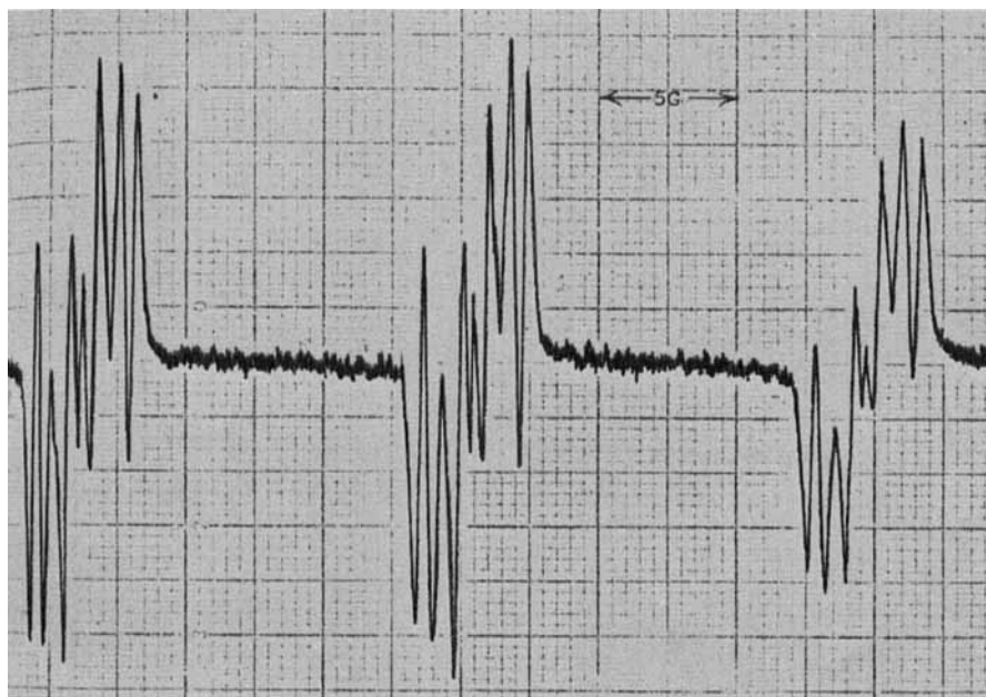
FIG. 9. ESR spectrum obtained in the reaction of the tetralin-DBPOX-BNO system at room temperature for 2 hr. [DBPOX] = 0.04 mole/liter; [BNO] = 0.02 mole/liter.
